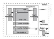
• Each column of photosensors has an amplifier associated with it (image can be transmitted above the noise).
