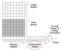
EMCCDS use similar structures to CCD's, but prior to being readout at the output node the charge is shifted through an additional register— the multiplication register— in which the charge is amplified.
