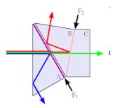
• After a light ray enters the first prism (A), the blue component is reflected by a coating (F1) at the AB interface (long wave-length bandwidth, high frequency).
